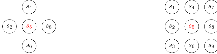
Figure 2: Local pixel neighborhood in 2D. The partially and fully connected neighborhoods are shown on the left and right respectively. The point s_5 in red is considered a local maximum if its value is larger than its neighbors.
